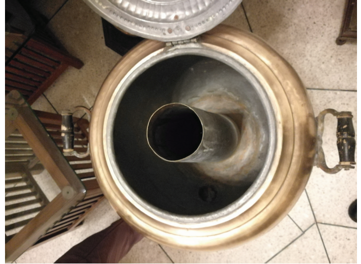
Fig. 5: The internal mechanism of the Traditional Indigenous Geezer at Chateau Garli is made of copper, Garli, H.P.
